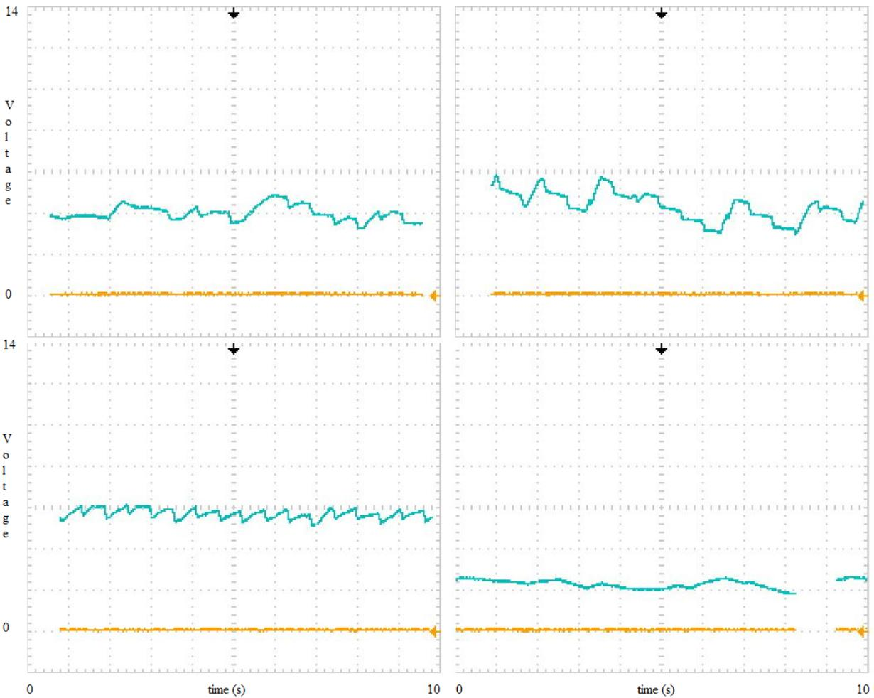
**Figure 16: WISP power traces for static ID. Blue trace is capacitor voltage and yellow trace is computation of packet (static ID is nearly instant). Distance from reader from top left to bottom right: 2', 3', 4', 5'**
