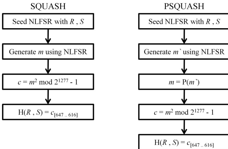
Figure 10: PSQUASH adds a permutation to the flow.
