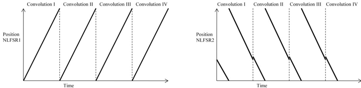
**Figure 3: NLFSR position needed to generate  $m$ .**
