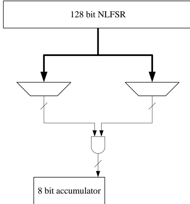
**Figure 9: A single NLFSR design proposed in [1].**
